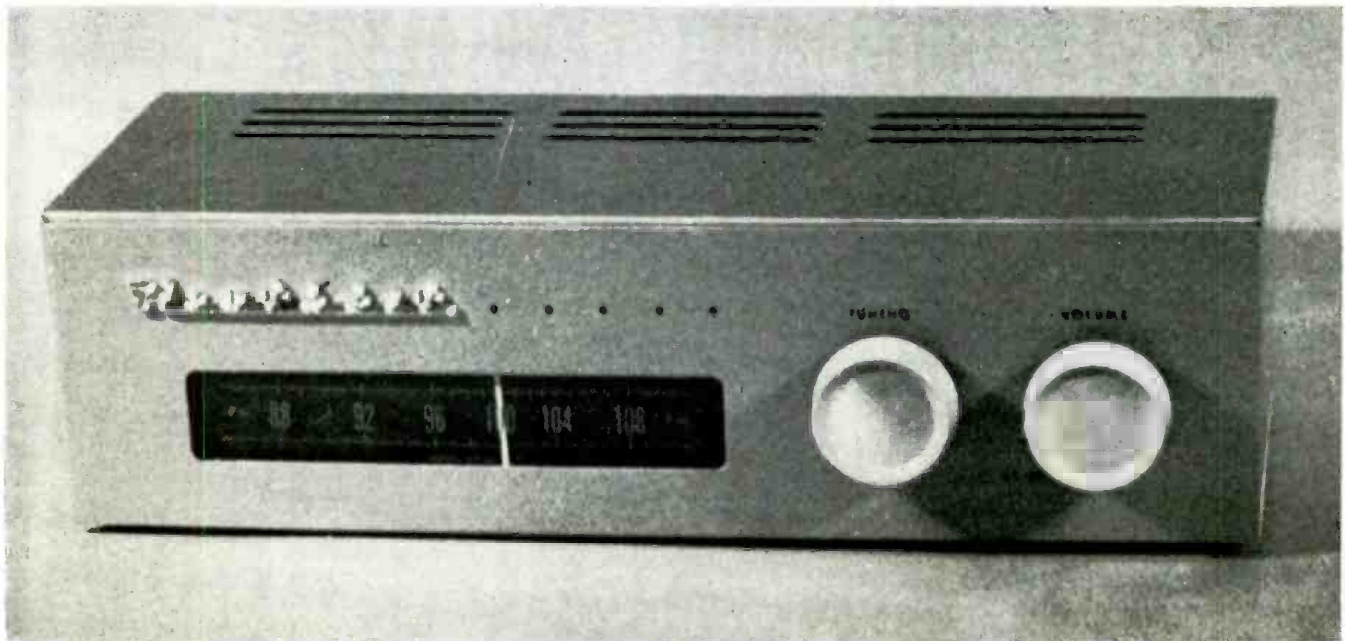
The finished tuner. Case is gold, knobs gray and the dial is edge lighted with green figures. All connections are made at the rear of the case. An output is provided which will operate a pre-amplifier and another, higher voltage output for attachment to any unit having a phono input. The connecting cable is furnished as part of the kit.
